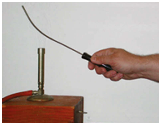
Sumber: www.physics.upenn.edu Gambar 4.6 Saat dipanaskan, bimetal melengkung.
